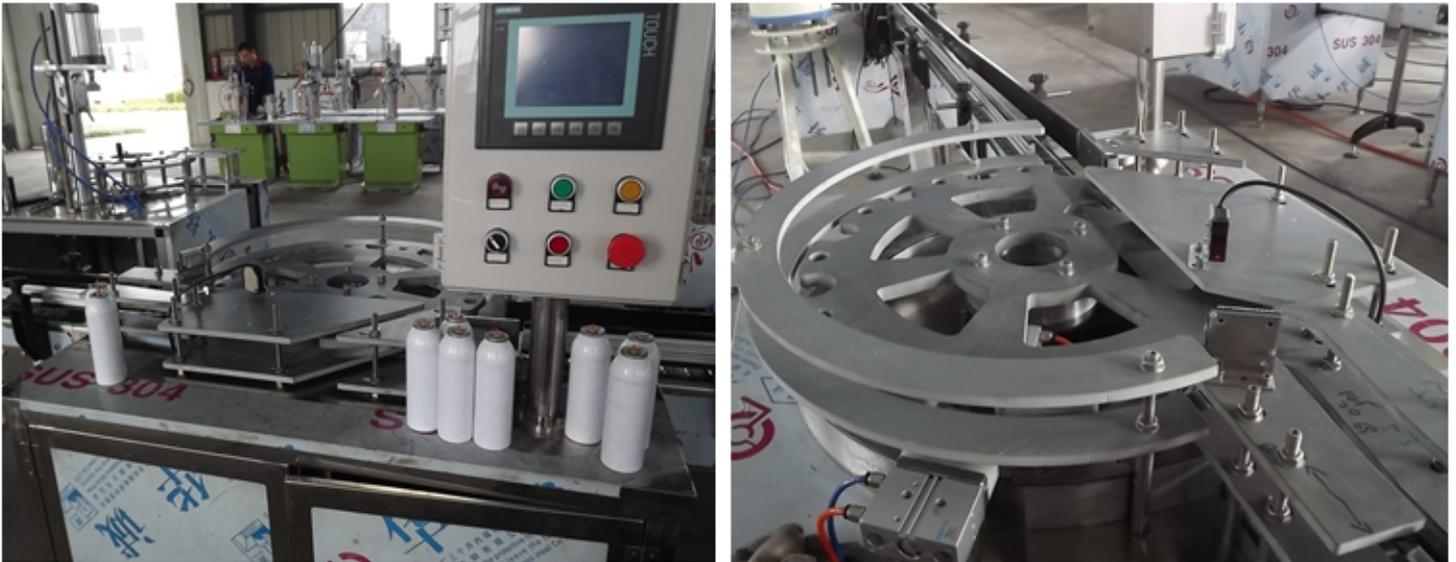
This machine can weight each can, and separate those weight are out of specification.
