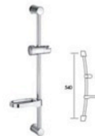
SD1016 ABS brackets, chrome plating ABS slider, chrome plating Stainless steel sliding bar Transparent soap dish Dimension: L:540, D:19
