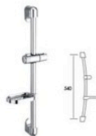
SD1011 ABS brackets, chrome plating ABS slider, chrome plating Stainless steel sliding bar Transparent soap dish Dimension: L:540, D:25
