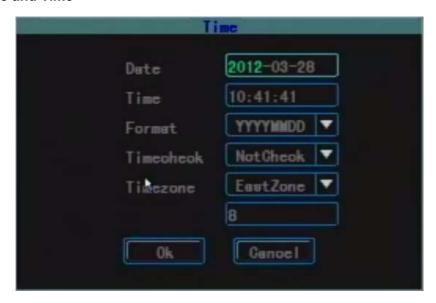
Enter the time page of the system, you can modify the time of the system and the time format. Note: the time can be modified when recording is stopped.
