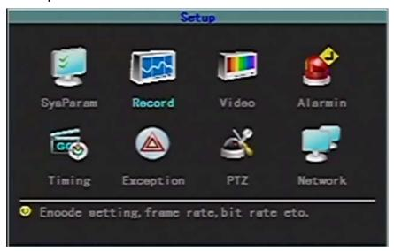
System setup includes Setup (system parameter), Record (recording setup), Image (image setup), Alarmin (alarm input), Schedule (schedule setup), Expection (expection handling), MTD (motion detection), PTZ (PTZ configuration) and Network.
