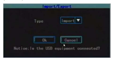
Used to export the system configuration to the USB disk, or import the system configuration from the USB disk, in order to facilitate configuring multiple devices in batch.
