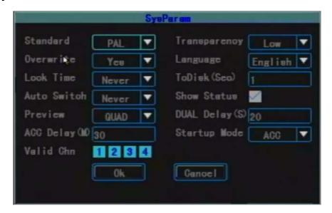
**Overwrite:** Select "Yes", when the HDD or SD card is full of recording, the system will overwrite the earliest video information to achieve the purpose of cycle recording. Select "No", when the HDD or SD card is full of recording, the system will not record any more; at this time, you can choose warning processing when the HDD is full in the menu of "Expection".
