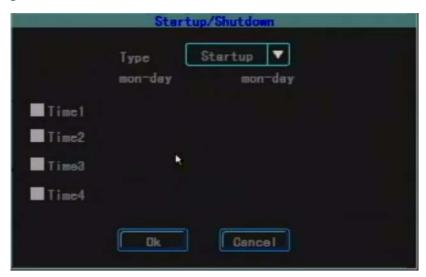
Used to set timing start or shutdown device. There are four time periods can be set and within each time period, you can set the time of start and shutdown every day.
