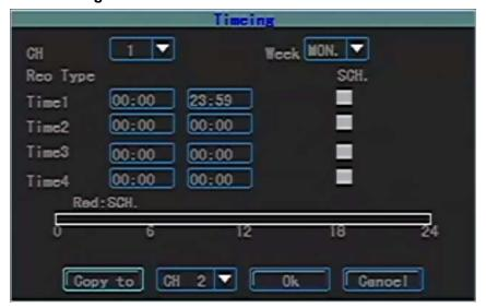
Used to set the time periods of timing recording, motion detection and alarm input recording.
