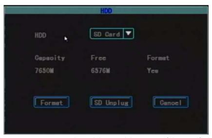
Check the current status, capacity and the remaining space of the specified HDD and if the HDD was formatted.
