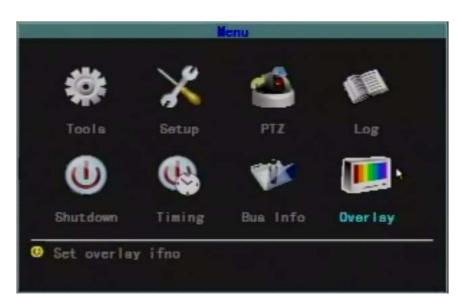
The menu includes Tools (management tools), Setup (system setup), PTZ (PTZ control), Log (log search), ShutDown (shutdown system), Timing (timing switch), BusInfo (bus information) etc..
