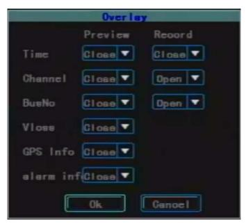
**Preview:** Used to set up whether to display time, channel number, bus number and if there is flashing prompting when video loss under preview mode. "Open" means display this item when preview while "Close" means not display this item on the interface when preview.
