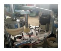
E.As other factory say their heating mold is flat,good for heating,but in fact,it is up to cup angle size,if the cup angle large,then use flat heating mold,if the cup angle size small,then need use round heating mold
