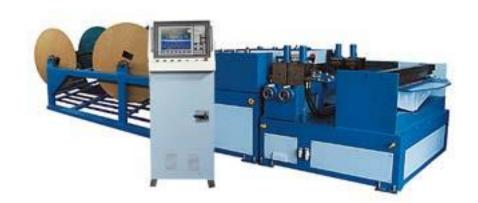
Line III consists of a decoiler, leveling & grooving rollers, hydraulic notching & punching machine, hydraulic shearer and hydraulic folder. The electrical control system uses a computer with a closed-loop servo-system to increase the precision and reliability of the line.
