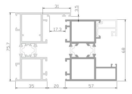
Section drawing of non-thermal break profile
