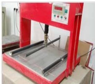
Bending Tester-for Hardness Inspection
