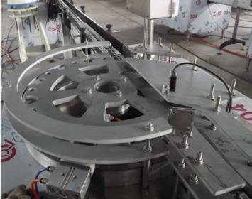
This machine can weight each can, and separate those weight are out of specification.
