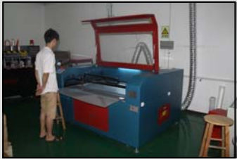
LGP(light-guiding plate) and RP(reflector plate) laser cutting
