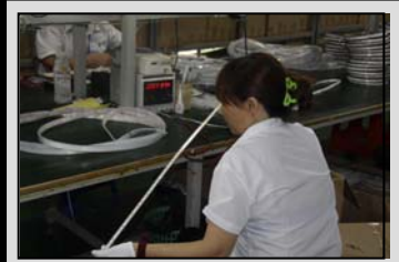
100% low-voltage test for LED antistatic performance
