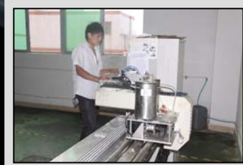
PU glue potting process
