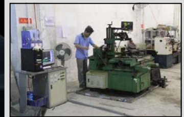
wire cutting machine
