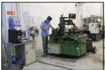
wire cutting machine
