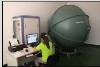
random inspection in photometric sphere
